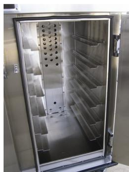
Heated compartment with vented plenum
